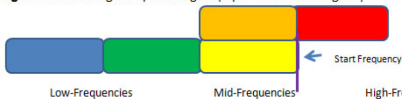
Figure 2B. Linear Frequency Transposition (Output of the Hearing Aid)
